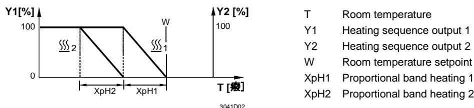
When two heating sequences are selected, the two outputs cannot be switched ON at the same time. Two outputs are switched ON separately with at least 10 seconds delay. In case of set-point change, the two heaters are allowed to switch OFF together.
